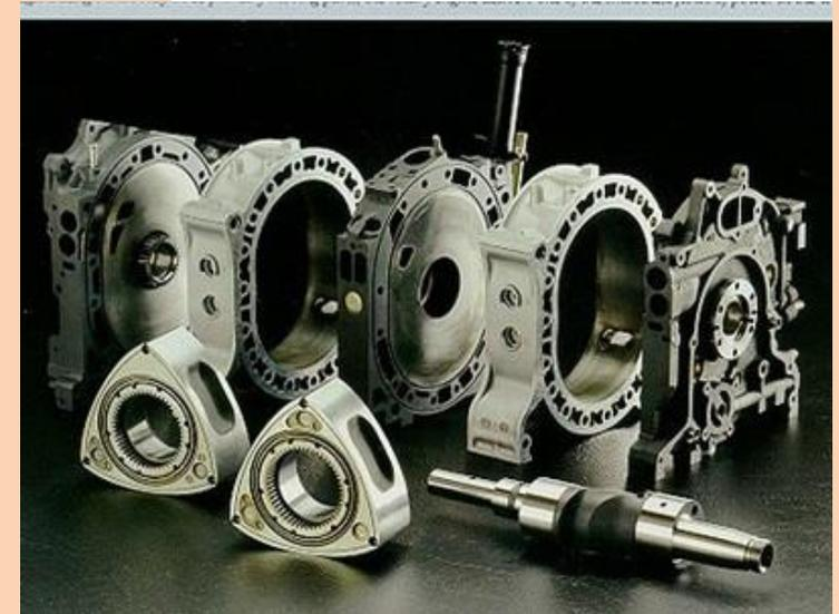
The Rotary/ Wankel burns as much as 20% more fuel than the conventional engine and is potentially a higher polluter, but its small size allows the addition of emission-control parts more conveniently than does the piston engine.
