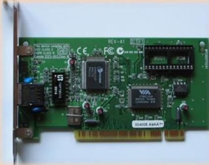
Computers have expansion slots on the motherboard to install adapter cards. The type of adapter card connector must match the expansion slot.
